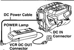
Connect AC Adaptor VCR DC OUT to Camcorder DC IN with supplied DC Power Cable.
